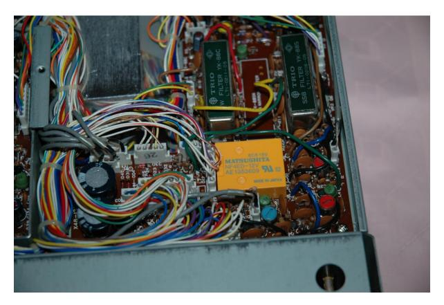
Having confirmed that the relay is functional, ensure you insert and screw down all the PCB screws. Do not overtighten them as you risk fracturing the board and ultimately damaging tracks on it.
