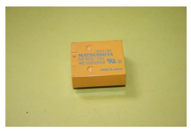
These relays can be bought online; it's a case of searching for them. It is a direct one for one swop. The pinout is exactly the same as the Omron it is replacing.
